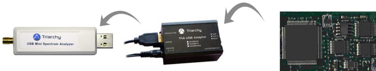
The TSA USB mini spectrum will connect to the USB2RS232, USB2RS232 will connect to embedden system
